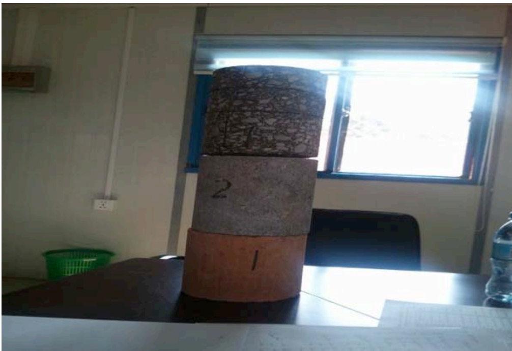
Quality control of airport pavement layers
